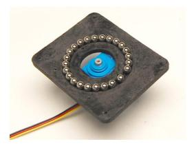
4. Center your servo and attach the pan top assembly to the pan bottom assembly. Check the alignment before proceeding.
