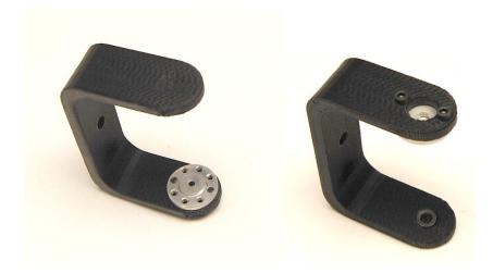
7. Insert the plastic nub (opposite of the servo hub) on the pan assembly into the tilt bracket. Bend the tilt bracket slightly to snap the hub on to the servo shaft.
