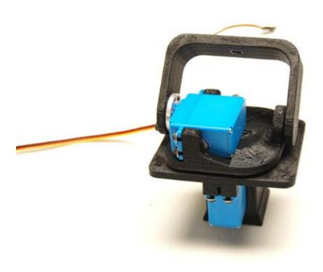
The Endurance R/C Pan and Tilt PT-2.1 base is a light weight pan and tilt system based around Hitec's line of waterproof servos: HS-646WP or the HS-5646WP. Featuring all around rigid ABS construction, the PT-2.1 base was designed for uses where moisture is an issue.
