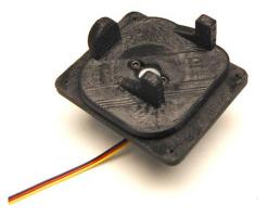
5. Attach a servo to the pan assembly with four 4-40 screws and washers.
